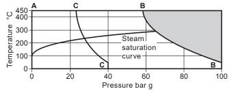
The product must not be used in this region or beyond the parameter of the PMA or TMA of the relative end connection.
