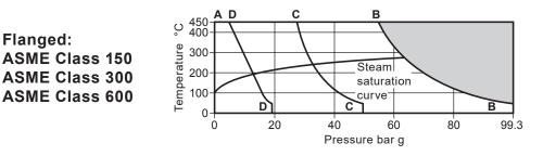
The product must not be used in this region or beyond the parameter of the PMA or TMA of the relative end connection.
